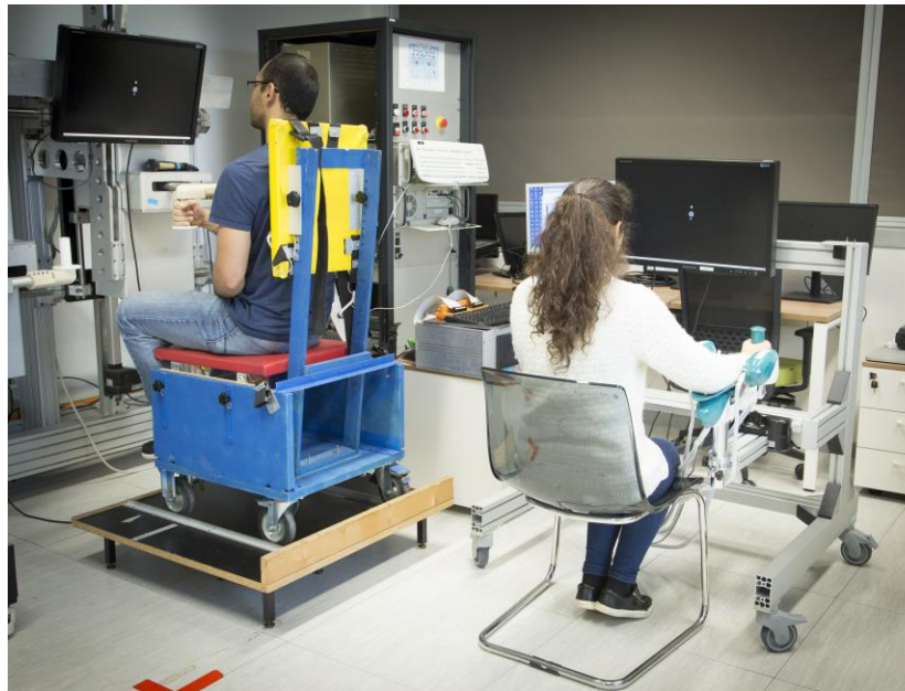
Figure 6-1: Experimental setup Braccio di Ferro – WristBot. The left handle of the Braccio di Ferro was substituted by the WristBot, in this way the subjects can share the same virtual reality while working in different haptic devices.
