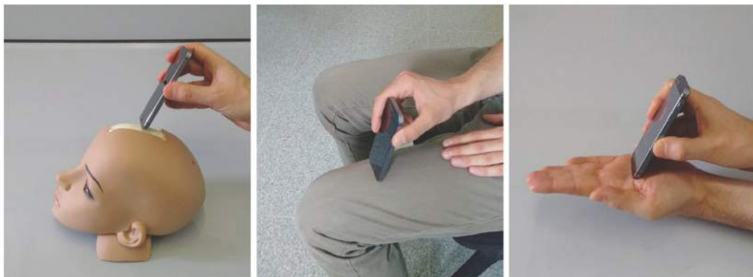
Figure 4.11: A common mobile phone can be used in order to simulate the probe positioning on any surface. From [PPM + 17]
