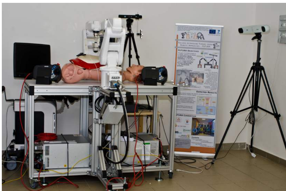
Figure 1.1: Setup for a robotic-assisted minimally invasive procedure. A surgical robotic platform, on the left, is used in conjunction with optical tracking systems, on the right and in the background.
