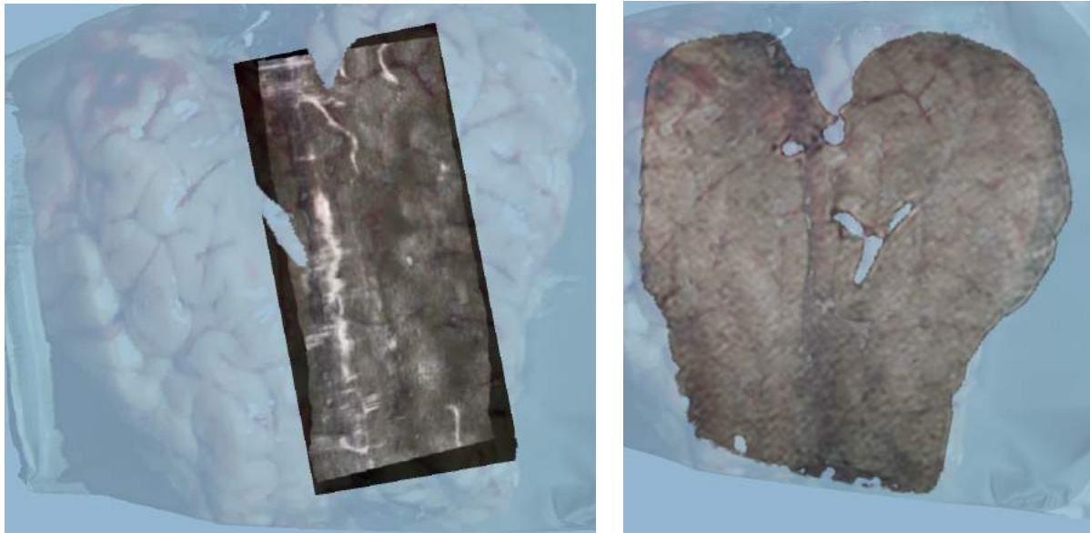
Figure 4.34: Fusion between US (left) or MRI (right) and phantom reconstructed surface. Camera point of view.
