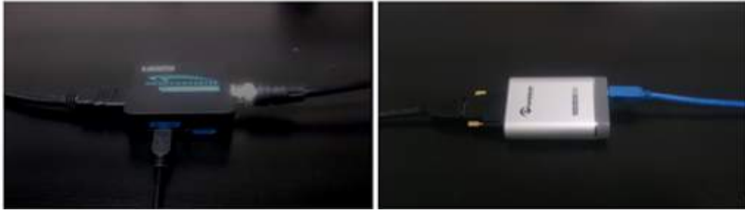
Figure 4.17: Acquisition pipeline hardware components, an HD-SDI to HDMI converter (left) and an Epiphan DVI2HDMI 3.0 Frame-grabber (right).
