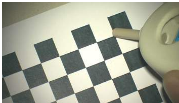
(c) Corner acquisition in the EMTS frame of reference by means of an EM pointer
