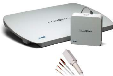
Figure 2.9: The NDI Aurora, an EMTS commonly used for medical tracking applications.
