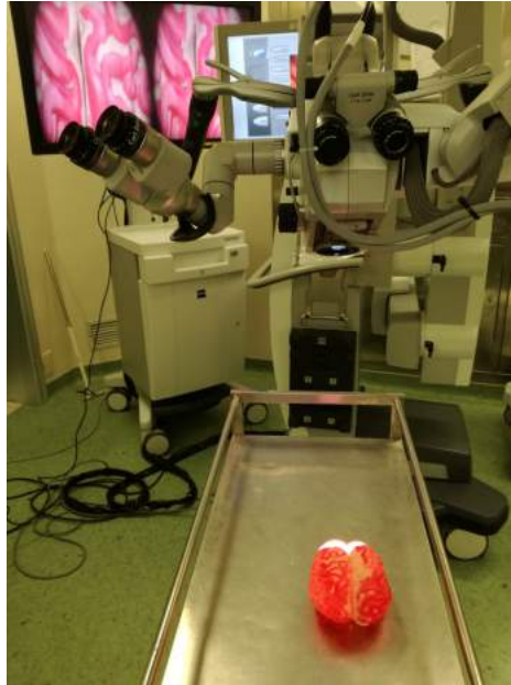
Figure 4.26: Experimental setup: the brain phantom is placed under the Pentero 900 surgical microscope, which is connected to the Trenion 3D HD system.
