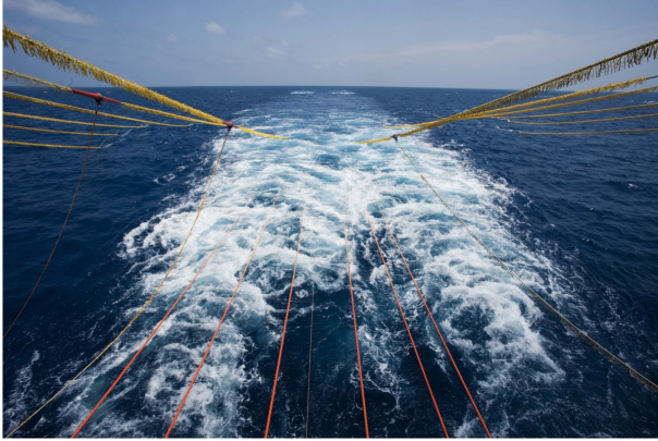
Fig. 1. Ship towed methodology for geotechnical surveying (picture courtesy of CGG).
