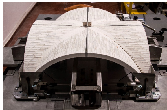
Figure 2.5. View of the built vault's model.
