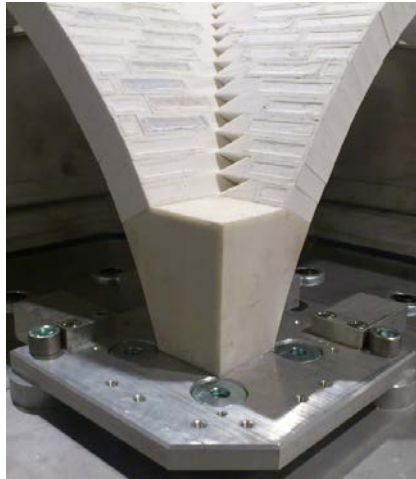
Figure 2.3. Interlocking between blocks at the intersection of the webs and vault's abutments.
