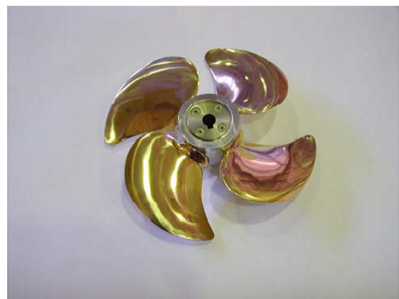
Figure 1: The RV Navigator XXI controllable pitch propeller.
