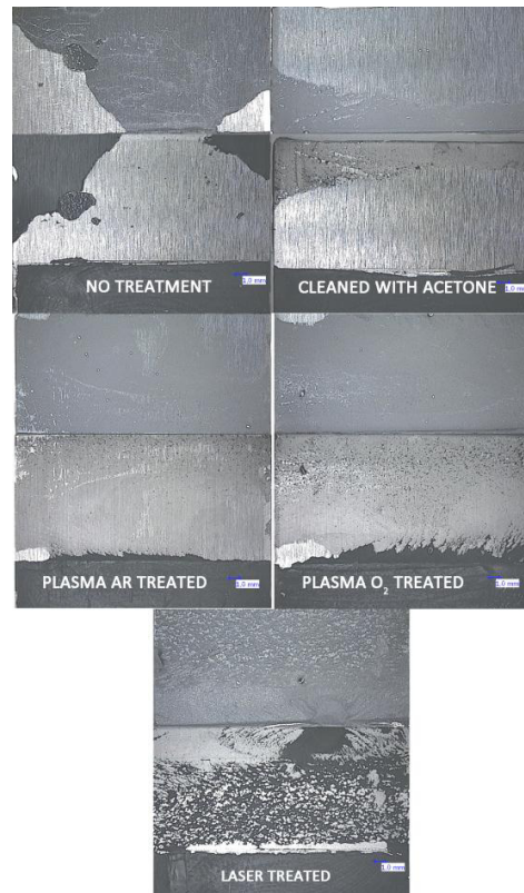
Fig. 7 Typical failure surfaces for different treatments.
