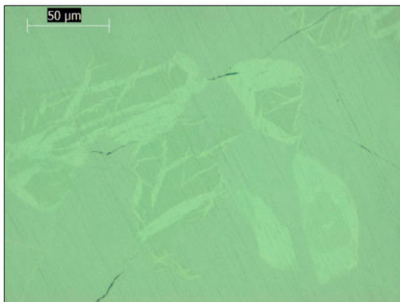
\text{Cu}_{76}\text{As}_6\text{Sb}_{18} [C6], annealed a 500°C. Phase not yet fully identified; compound: \text{Cu}_{11}(\text{As,Sb})_3 .
