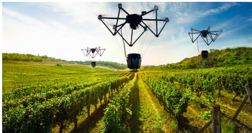
Fig. 1. Rendering of UAV equipped with bucket over vine rows
