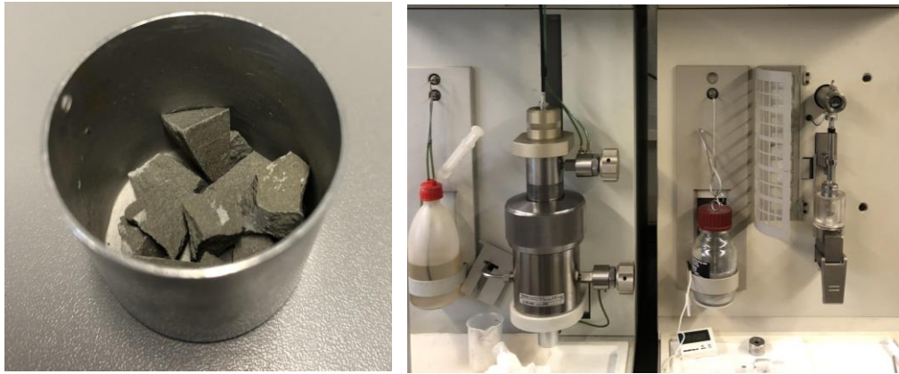
Figure 3: a) Sample holder together with Specimen Fractures tested under MIP and b) Mercury intrusion porosimeter Thermo Scientific Pascal 140 and 440.
