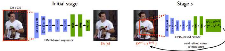
Figure 3.4: DeepPose architecture (source: [Toshev and Szegedy, 2014]). Convolutional layers in blue and fully connected ones in green.
