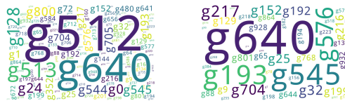
Figure 4.6: BOW (left) and tf-idf (right) word cloud visualization of an infant's temporal network. The size of configuration names is proportional to their weights in the corresponding representation. Note that the configuration g_{512} is either very frequent or rare in the collection of infants networks and therefore it has weight equal to 0 in the tf-idf representation.
