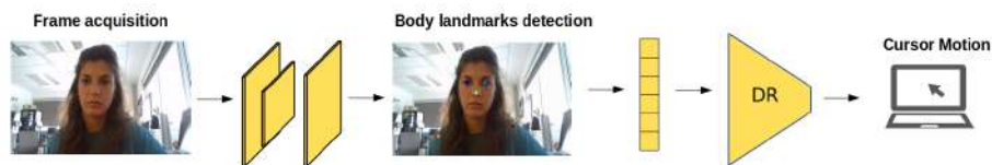
Figure 7.8: Summary of the BoMI pipeline. The image acquired by the computer webcam is fed through the trained network to detect the body landmarks. Then, a dimensionality reduction (DR) algorithm is applied to the landmarks' signal to obtain the coordinates of the computer cursor.
