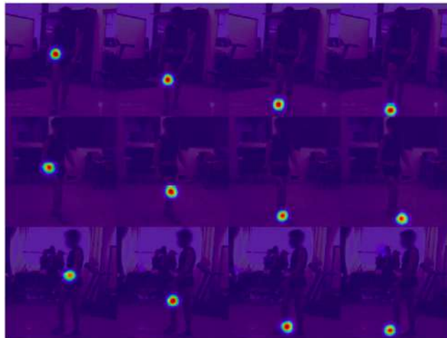
Figure 4.1: Example of probability maps for different body landmarks. Red and blue correspond to high and low probability respectively.
