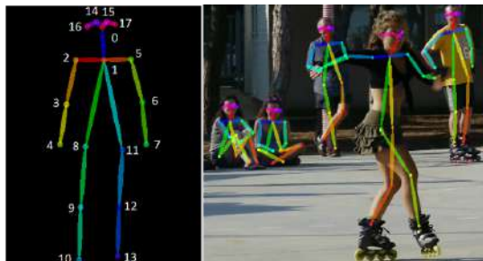
Figure 3.1: Examples of human skeleton with the meaningful body keypoints (left panel) and pose estimation from an RGB image (right panel). Source: [Cao et al., 2017].
