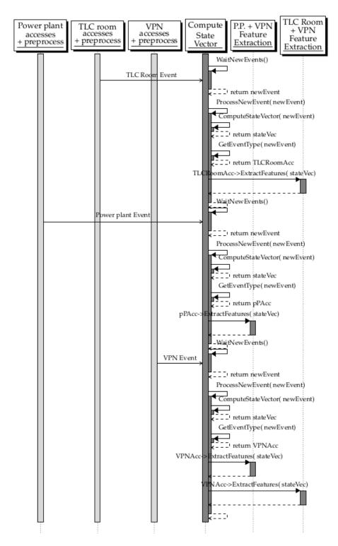
Figure 6.6 Sequence diagram showing the complete first part of the implemented system with three log sources and two extraction blocks
