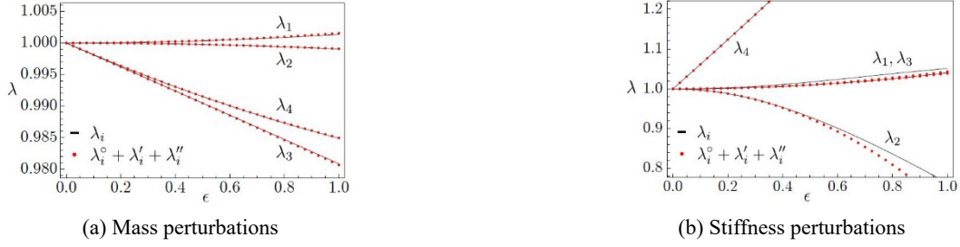
Fig. 2 Comparison between the exact and approximate eigenvalue loci (normalized with respect to the unperturbed eigenvalue) versus \epsilon -proportional perturbations of (a) the mass matrix; (b) the stiffness matrix of the deformable diaphragm (parameters \beta = \frac{2}{3}, \chi^2 = \frac{1}{4}, \kappa_s = \frac{1}{3}, \Sigma_\rho^2 = 9, \Sigma_{\kappa x} = 2, \Sigma_{\kappa y} = 1, \Delta_{\rho x}^2 = \frac{1}{4}, \Delta_{\rho y}^2 = \frac{1}{9}, \Delta_{\kappa x} = \frac{1}{4}, \Delta_{\kappa y} = \frac{1}{5} )
